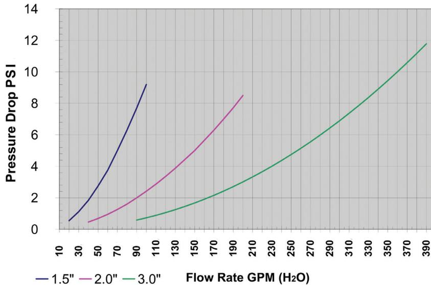
Tests on 1½", 2" and 3" hoses equipped with Bayloc™ cam and groove dry disconnect couplers and adapters show only a very modest pressure drop at various flow rates. As an example, for a 2" hose at a flow rate of 90 gallons per minute, the pressure drop is just 2 PSI (pounds per square inch).
