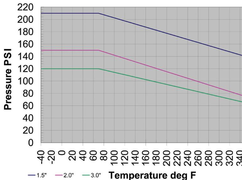
The higher the temperature of the media being transferred, the greater the likelihood of pressure de-rating. High-temp substances being transferred, such as asphalt and pitch, experience the largest pressure de-rating – in the case of a 3" hose, declining from 120 PSI to approximately 70 PSI.
